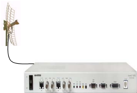
An Aurora 2400 1xT1/E1 DSSS Radio Terminal
